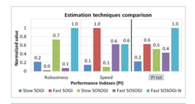
Fig. 3 - Normalized comparison of the angular quantities estimators in terms of robustness and fastness. A global combined normalized index is reported in PI tot.
