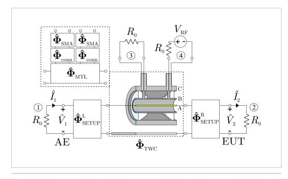
Fig. 3 - Distributed-parameter model of the TWC mounted on the CF. The TWC model is detailed in the up-left panel.
