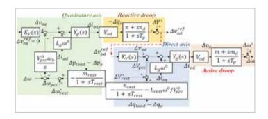
Fig. 2 - Dynamical model of the converter under droop regulation.
