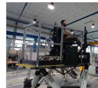
Fig. 3 - OPT-IN system integrated in a motion platform during a test
