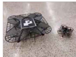
Fig. 1 - ANT-X and CARRIER-1 drones employed for testing vision-based Air-to-Air Automatic Landing. The small drone is equipped with a monocular camera, while the larger drone is equipped with a fiducial marker.
