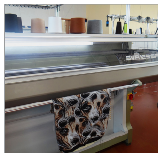
Fig. 2 - Jacquard fabric produced by the Shima Seiki knitting machine. Maglificio Pozzebon. Photo by A. Alves Santos.
