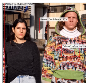
Fig. 3 - Technology test with YOLO. The person wearing Cap_able is not classified as a person by Artificial Intelligence. Photo by Rachele Didero.
