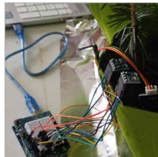
Fig. 1 - Multiparametric detection applied on indirect VGS for the detection of Temperature, Relative Humidity, Pressure, Altitude, Soil Humidity, Lux.
