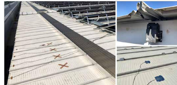
Fig. 1 - Experimental setup to monitor standing seam panels' longitudinal thermal expansion using wire displacement transducers and surface temperature sensor.
